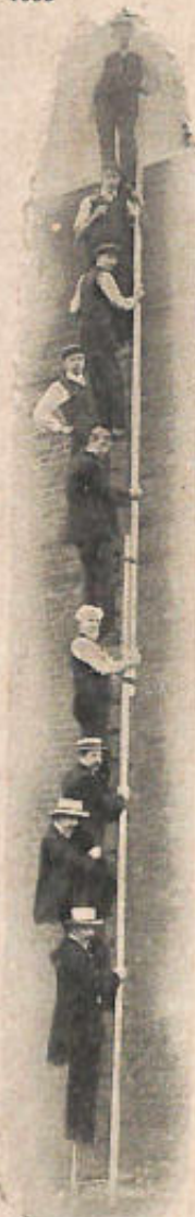
Slingsby-Steelback Patent Extension Ladder.
