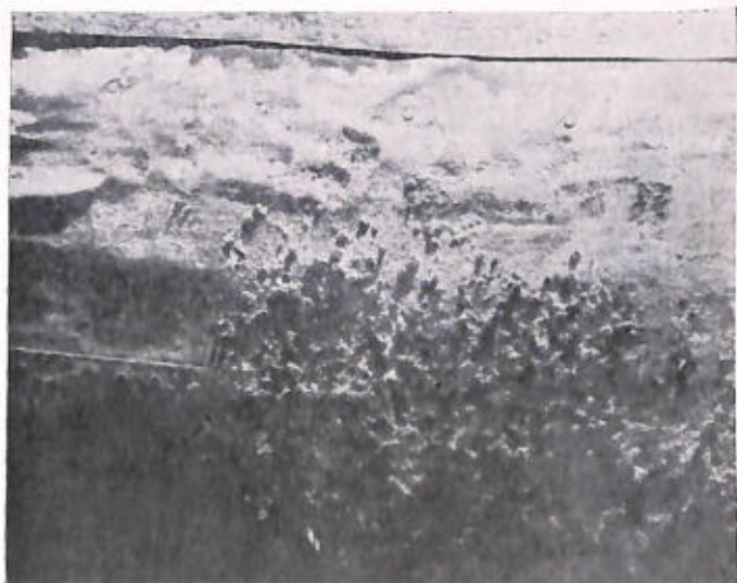
Fig. 2. Barnacle fouling on copper sheathing.
