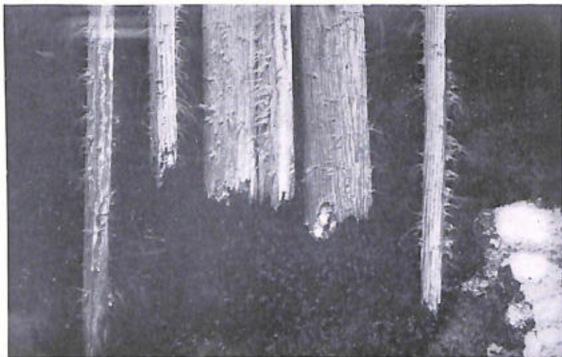
THE SHIPWORM ( Teredo navalis ) is enormously destructive to the timbers of wharves and the hulls of vessels. Pieces of wood completely filled with shipworms are often to be seen in the tanks of the Aquarium
