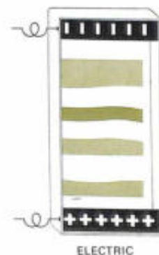
Plant proteins are separated by electrophoresis. The protein is first dissolved and then applied to the centre of a strip of wet paper (dark line above). When an electric current passes through the paper, the sample separates into bands, as positive and negative particles move towards the two poles at different rates of speed.
