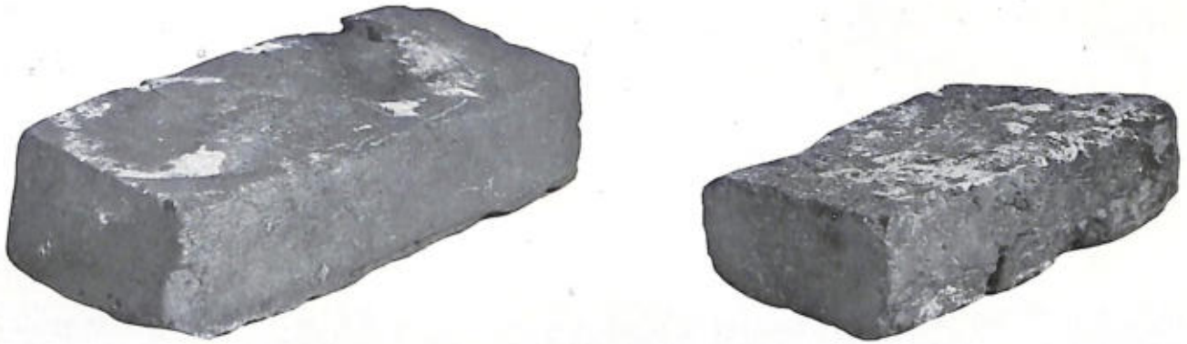
Figure 53.—VIRGINIA BRICK from Structure B (left) 9 by 4 by 2\frac{1}{4} inches. Right, small brick from Structure F, probably imported, 7\frac{1}{4} by 3\frac{1}{2} by 1\frac{1}{4} inches. Perhaps one of the 630 bricks brought on the Marigold by Captain Roger Lyndon and purchased by John Mercer.
