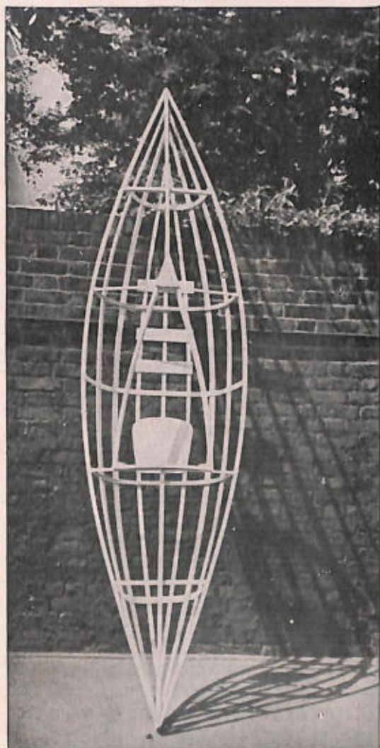
This photograph shows the construction of the framework of a rigid eleven foot single canoe of the Tyne Kit type.
