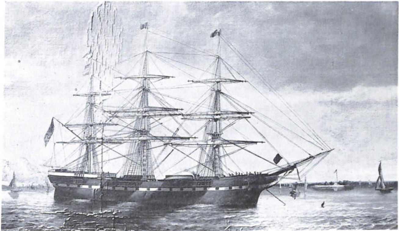
PACKET SHIP, BUILT IN 1855 AT NEW YORK CITY BY WILLIAM H. WEBB FOR THE BLACK BALL LINE, the Neptune . She was wrecked about 1877. Her register dimensions were 191' x 40' x 28', 1,406 tons. From a painting (USNM 310852) in the Watercraft Collection. (Smithsonian photo 44691.)
