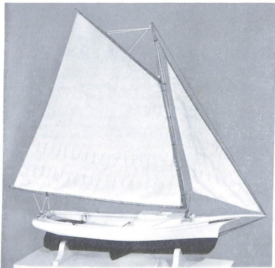
MUSCONGUS BAY SLOOP, 1880. A type of centerboard boat used on the Maine coast in the vicinity of Muscongus Bay. It was a forerunner of the later and better known Friendship sloop. Rigged model USNM 55795. (Smithsonian photo 45605-c.)
