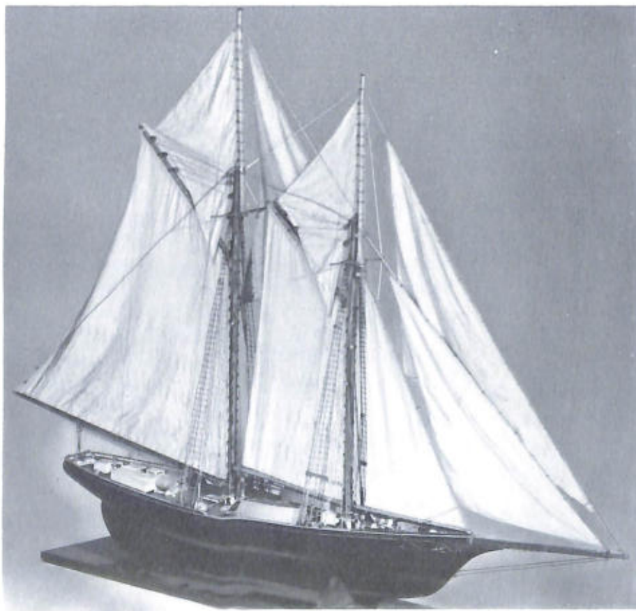
COD FISHING SCHOONER John J. Flaherty , 1899, an excellent example of the last clipper-bowed schooners built for the fisheries. Rigged model USNM 285030. (Smithsonian photo 44693.)
