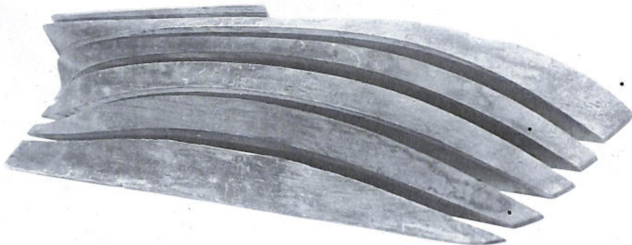
STANDARD LIFT HALF-MODEL WITH FASTENERS REMOVED AND THE LIFTS SLIGHTLY SPREAD. A quarter deck rail lift is shown. This model, in the author's collection, is of a Connecticut schooner, name unknown, of the pilot-boat type, built at Westbrook, Connecticut, about 1825-30. (Smithsonian photo 45608-1.).
