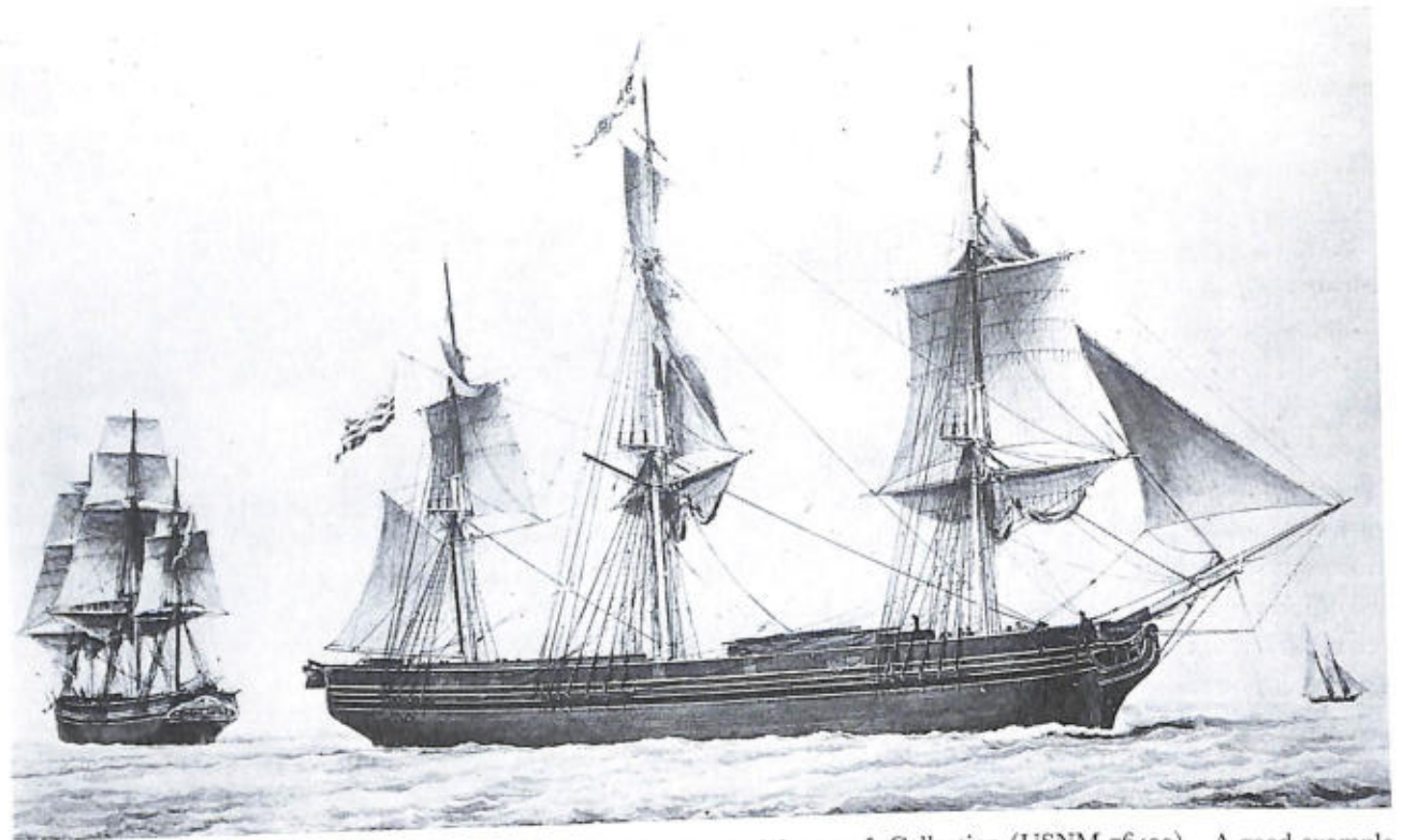
MERCHANT SHIP Bazaar , from a French print in the Watercraft Collection (USNM 76499). A good example of an American freighting ship of the period 1825-45, she was built at Medford, Massachusetts, in 1834 and employed in the European trade. Her register tonnage was 490, old measurement. (Smithsonian photo 44638-g.)
