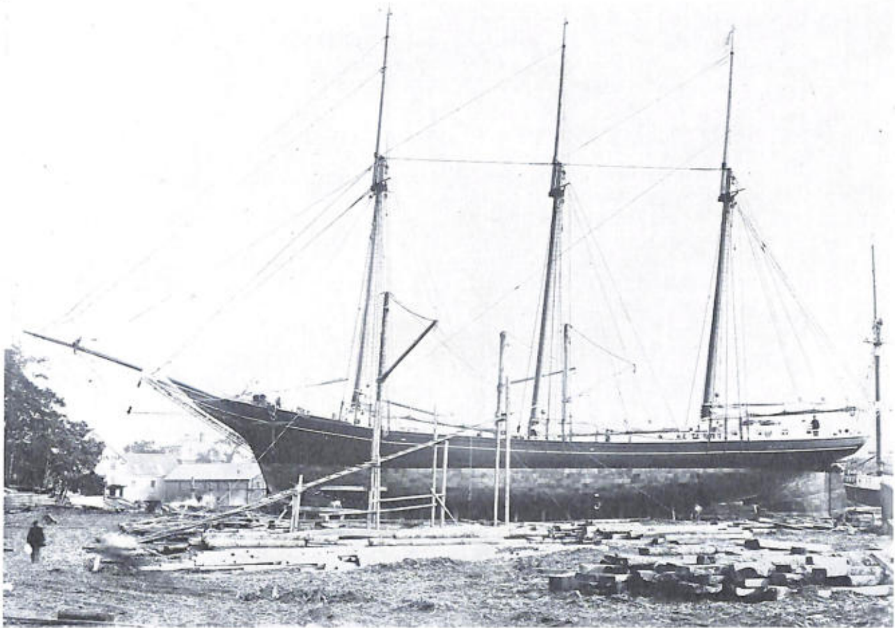
THE 3-MASTED SCHOONER J. S. Hoskins , built by the New England Ship Building Company, Bath, Maine, for Emerson Rokes, of Baltimore, Maryland. Launched October 26, 1886, her register dimensions were 193.9' x 34.2' x 11.5', 411.56 gross tons. Her captain was Joshua A. Rich. (Smithsonian photo 44588.)
