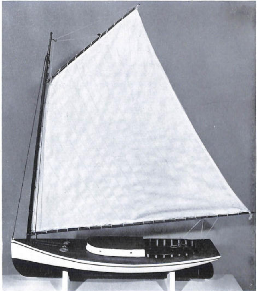
FISHING CATBOAT of the type used on the Massachusetts and Rhode Island coast, 1875-80. Rigged model USNM 25026. (Smithsonian photo 45605-h.)
