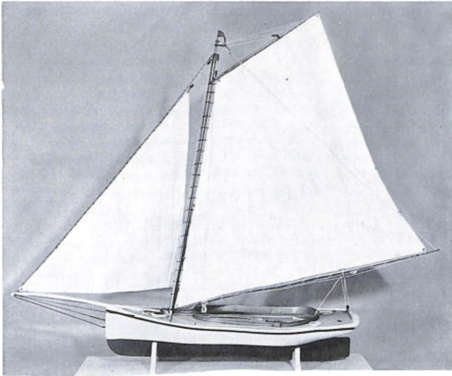
CENTERBOARD NOANK SLOOP of the type used in the lobster fishery on Long Island Sound, 1875-1900. Rigged model USNM 26809. (Smithsonian photo 45605-d.)
