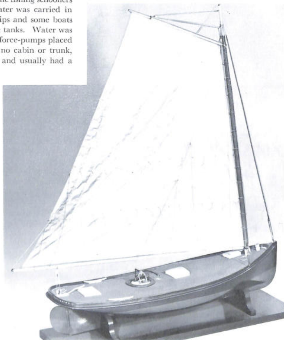
GLOUCESTER WATERBOAT Aqua Pura , built in 1883. This rigged model, USNM 56973, shows very well the typical deck arrangement and rig. (Smithsonian photo 44693-m.)
