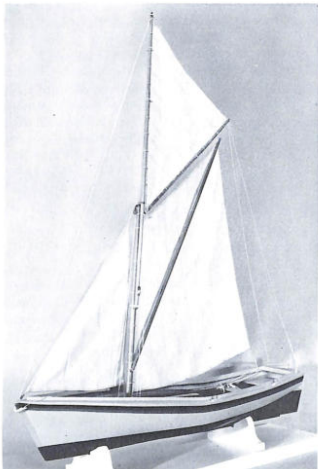
CROATAN FISHING BOAT used for shad fishing in the vicinity of Roanoke Island in the North Carolina Sounds, 1880's and 1890's. Rigged model USNM 76255. (Smithsonian photo 45606-a.)
