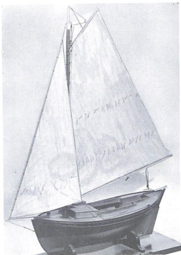
QUODDY BOAT Yankee Hero , 1889. Rigged model USNM 76266. An average size boat of her type, she was built to carry sardines from the weirs to the canneries. The builder's half-model of this boat is USNM 76293. (Smithsonian photo 44696-g.)
