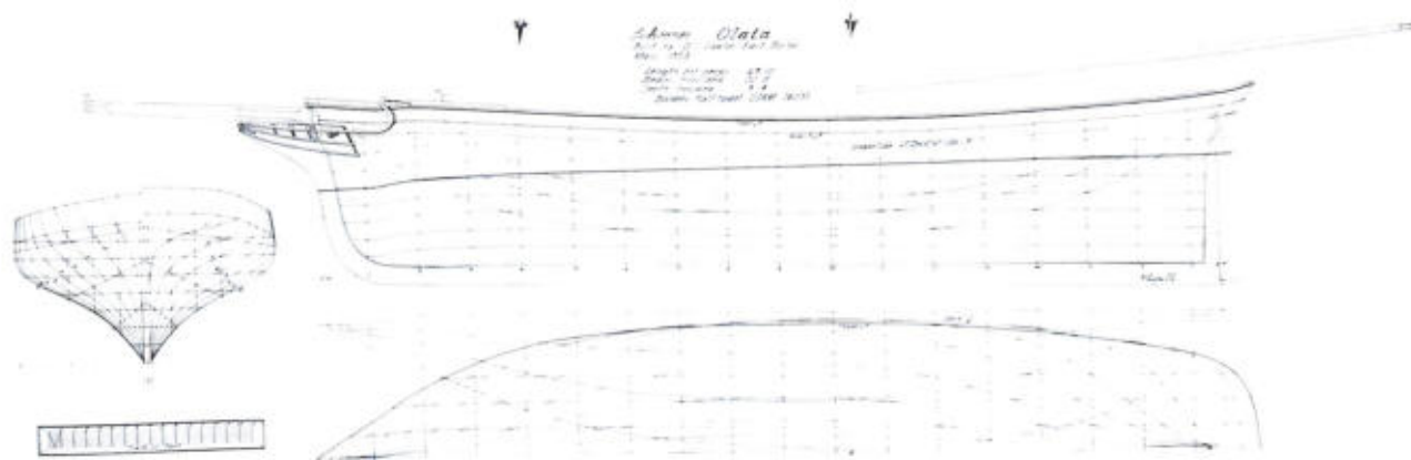
LINEs OF THE PILOT SCHOONER AND YACHT Olata , built at East Boston, Massachusetts, in 1853. Taken off the builder's half-model USNM 76035.
