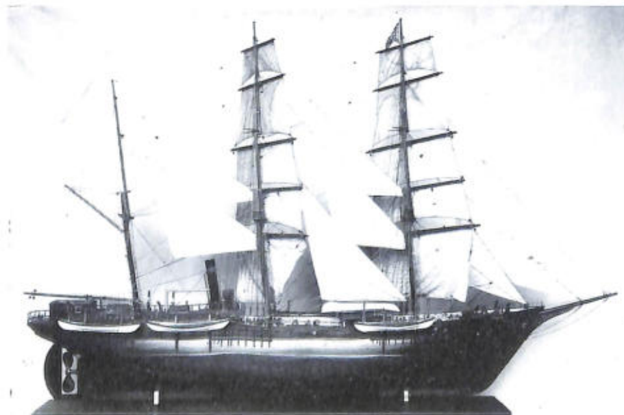
WHALING STEAMER Orca , built at San Francisco, California, in 1882. The largest of her type when built, and most completely fitted, her register dimensions were 177' x 32'6" x 18'11", 462.39 net tons, 280 horsepower. Abandoned off Point Barrow, Alaska in 1889. Rigged model USNM 76237. (Smithsonian photo 26758-h.)
