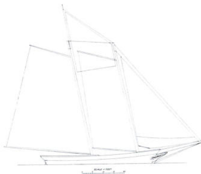
SAILMAKER'S PLAN for the sharpshooter fishing schooner Romp built at Essex, Massachusetts, 1847. From a drawing, made for the U.S. Fish Commission, in the Watercraft Collection.
