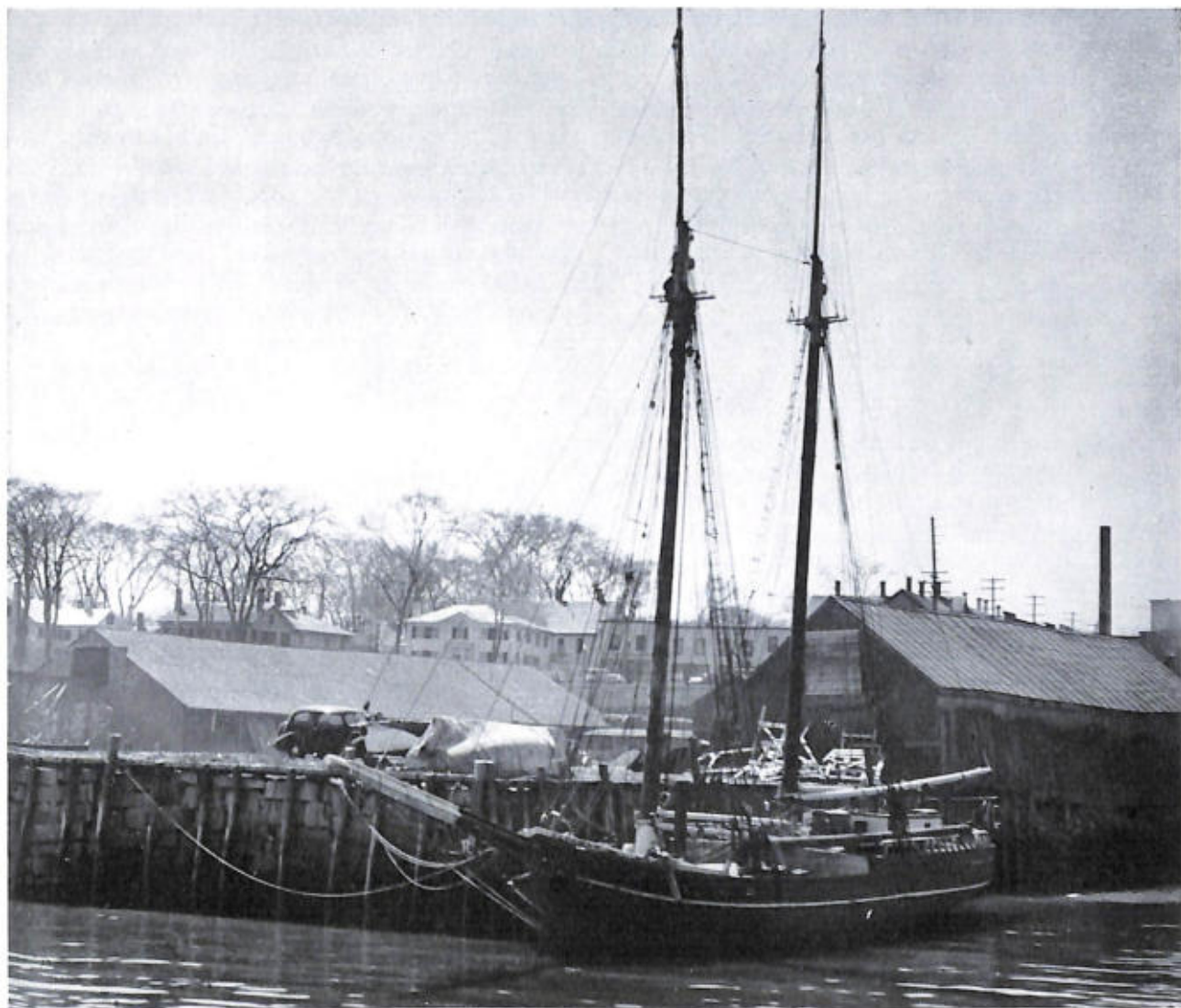
COASTING SCHOONER Bloomer , at Belfast, Maine, in 1936. Built at Eden, Maine, in 1855, her register dimensions were 64.3' x 21.8' x 6.2', 51 gross tons. (Smithsonian photo 45785-a.)
