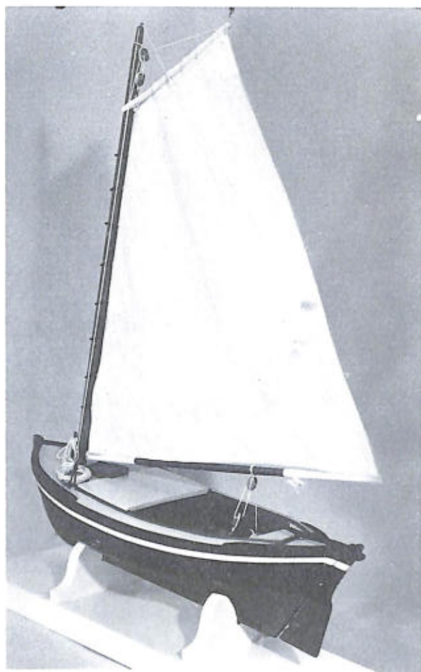
SARDINE CARRIER of the smaller size in use at Eastport, Maine, in the 1880's. This type was known as a quoddy boat, after Passamaquoddy Bay, Maine. Rigger model USNM 12099. (Smithsonian photo 45605-j.)
