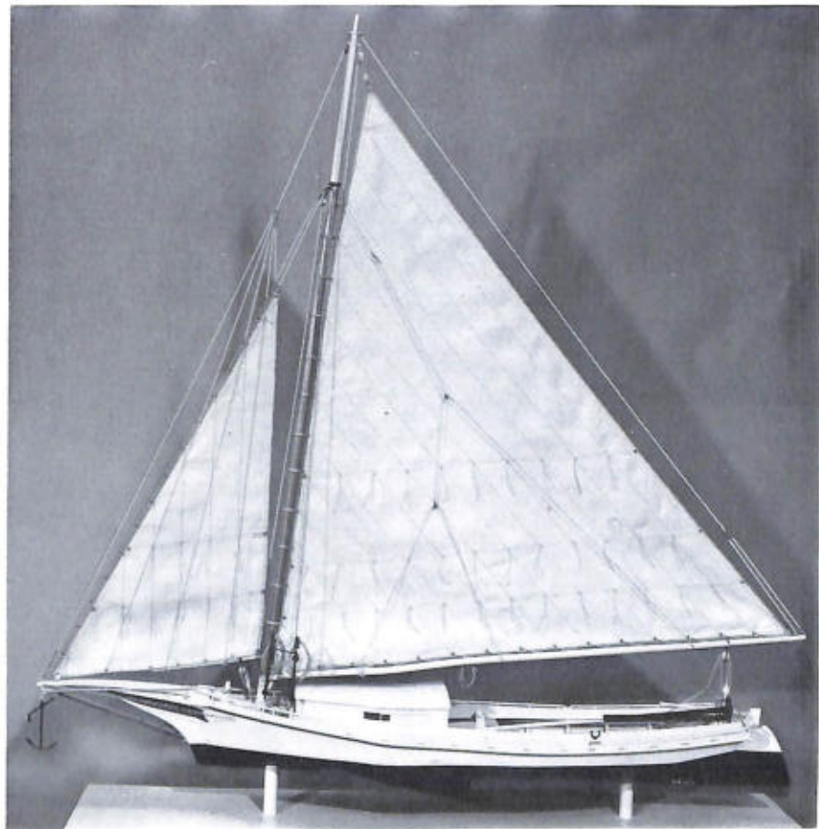
CHESAPEAKE BAY SKIPJACK, or "crab scraper," Jesse Willard , built near Deal Island, Maryland, in 1915. Rigged model USNM 316629. (Smithsonian photo 45606-g.)
