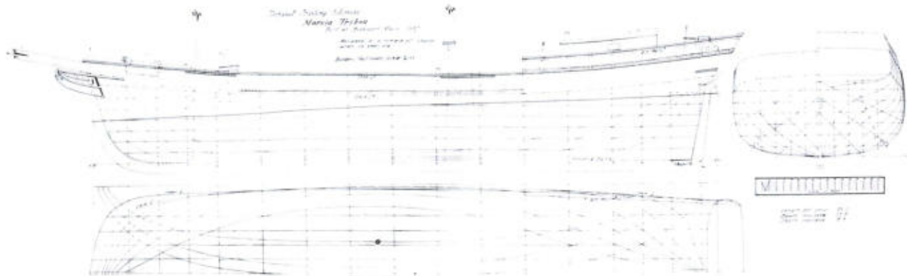
LINES OF THE SQUARE-TOPSAIL COASTING SCHOONER Marcia Tribou built at Bucksport, Maine, in 1847 for the lumber trade. Taken off the builder's half-model USNM 76104.
