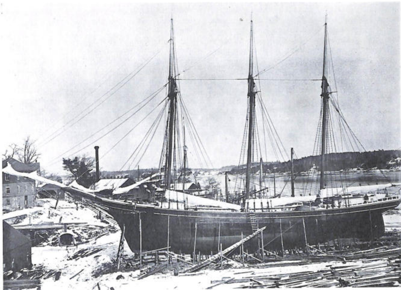
THE 3-MASTED SCHOONER Cactus , built at Bath, Maine, in 1890. Her register dimensions were 149.4' x 34.7' x 12.8', 534.59 gross tons. (Smithsonian photo 37382-a.)
