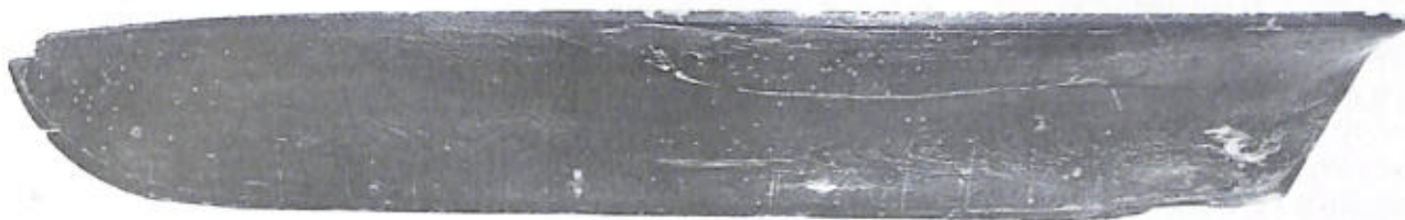
BUILDER'S BLOCK MODEL (USNM 316628) OF THE PRIVATEER Snap Dragon (see p. 88). Made before 1812 and the oldest half-model in the collection, it was shaped from a solid block of wood. To raise the deck level and thus alter the depth, a thin plank, or lift, was added to the top. Lines were probably taken off with a lead bar by the builder. (Smithsonian photo 45608-m.)
