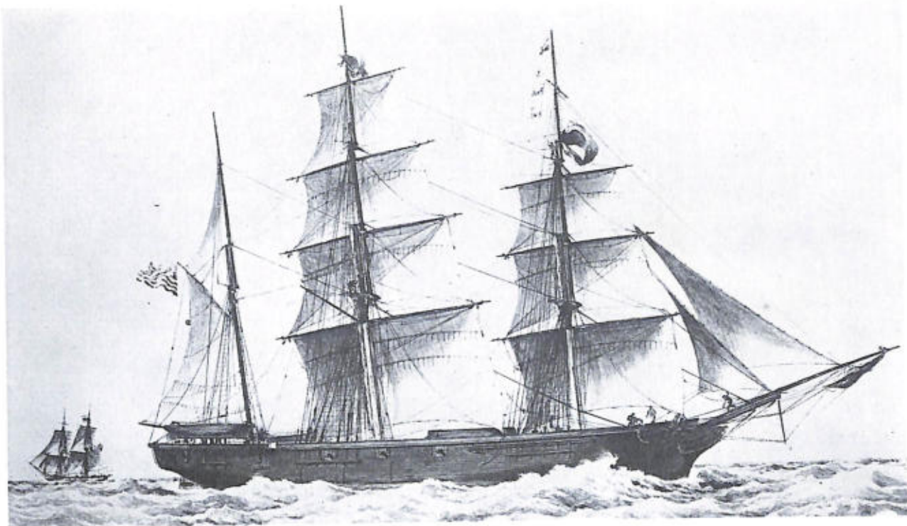
THE CLIPPER BARK Race Horse , from a French print in the Watercraft Collection (USNM 159926). She was built in 1850 by Samuel Hall, at East Boston, Massachusetts, for Boston owners. A medium clipper of small size and a good sailer, her register dimensions were 125' x 30' x 16', 530 tons. (Smithsonian photo 44638-j.)
