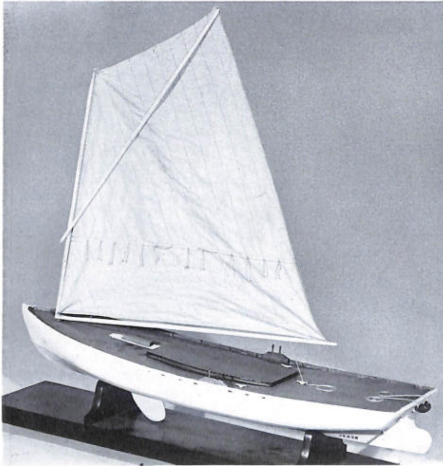
EGG HARBOR MELON-SEED GUNNING SKIFF from lower Barnegat Bay, New Jersey. Rigged model USNM 25658 showing a typical boat of this type. (Smithsonian photo 44697-a.)
