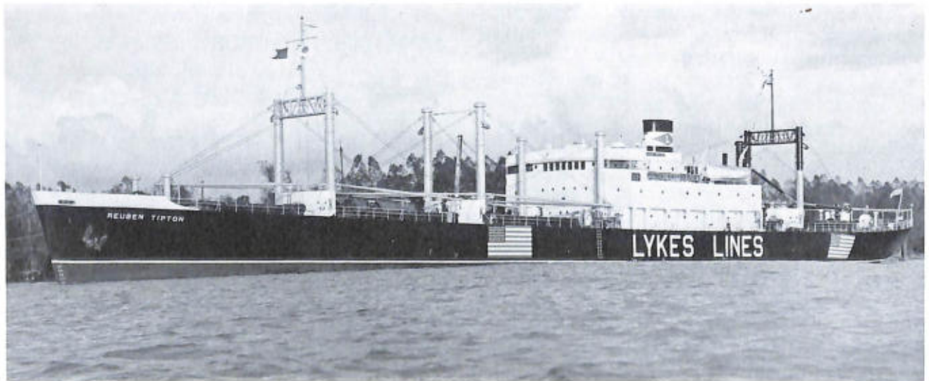
AMERICAN MERCHANT SHIP, CLASS C1-B, MODIFIED FOR USE OF A PRIVATE OPERATOR. Rigger model USNM 313021 shows the basic design of the class. (U.S. Maritime Administration photo 2106.)
