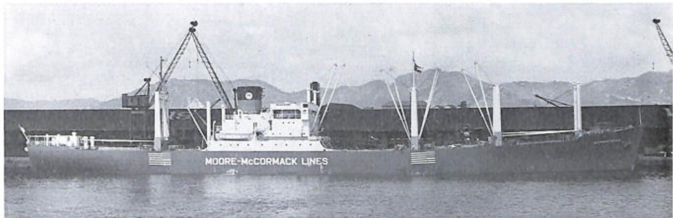
AMERICAN MERCHANT SHIP, CLASS C-2, MODIFIED FOR USE OF A PRIVATE OPERATOR. Many of this design were employed in war service. Rigged model USNM 313024 shows the basic design of the class. (U.S. Maritime Administration photo 1416.)
