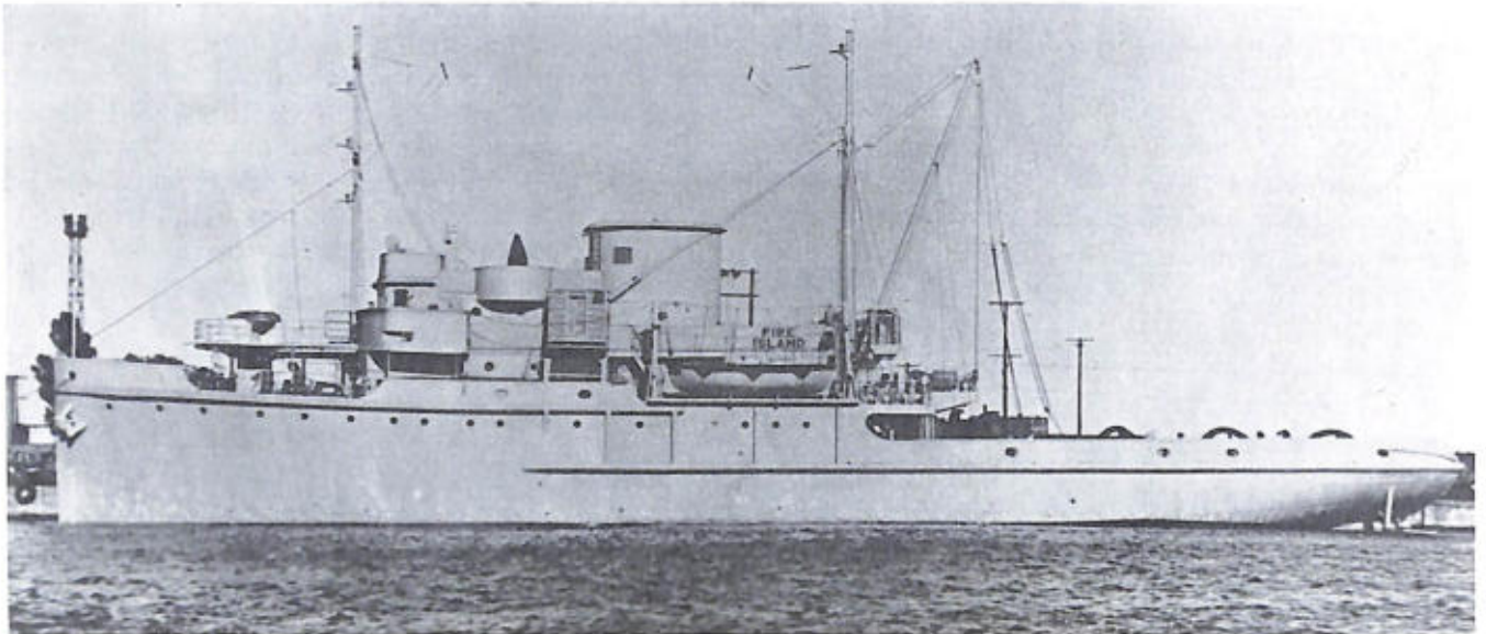
SEAGOING TUG AND SALVAGE VESSEL, CLASS V-4, FITTED FOR WAR SERVICE. Rigged model USNM 313020 shows basic design of class. (U.S. Maritime Administration photo 5059.)
