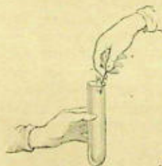
Fig. 14. — The match lights in the oxygen, this gas then keeps up combustion.
