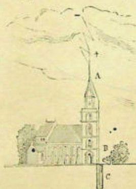
Fig. 74. — If a thunder bolt falls, it follows in preference the chain AB and is lost in the earth C.
