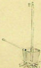
Fig. 18. — Thermometer immersed in boiling water. — Temperature : 100°.
