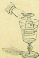
Fig. 3. — The water only mounts to A, the space B, is filled up with air, which is a gas.
