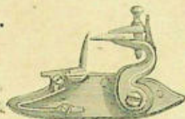
Fig. 6. — Lock of a gun. It is the spark which inflames the powder.
