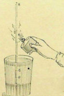
Fig. 12. — The tube being closed at A, the air in the interior expands under the influence of heat, and causes the water to descend from C to D (expansion of gas).
