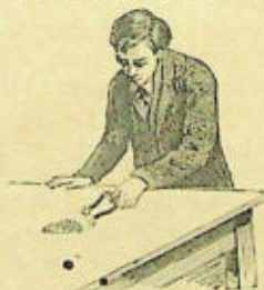
Fig. 6. — The magnet attracts all the filings, and leaves the sulphur: mixture .
