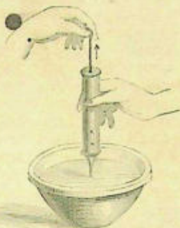
Fig. 120. — The water in the basin under the atmospheric pressure rises in the little ear syringe.
