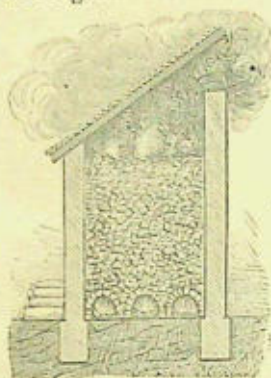
Fig. 7. — An oven for burning plaster. — Gypsum submitted to a great heat becomes plaster.
