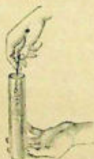
Fig. 20. — The match goes out in the nitrogen. So this gas does not support combustion.
