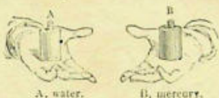
Fig. 100. — The density of water A (weight of the same volume) being 1 that of mercury B is 13.5.
