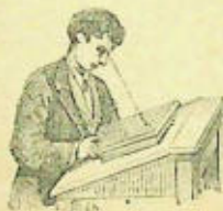
Fig. 33. — The lines of the book, in passing from the glass into the air, appear deviated: simple refraction.
