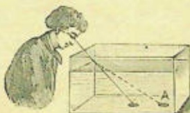
Fig. 32. — The luminous ray is broken on leaving the water, and causes the penny to be seen at A in advance of the spot where it actually is (refraction).
