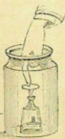
Fig. 9. — When the glass is at the bottom, the air is compressed at B.
