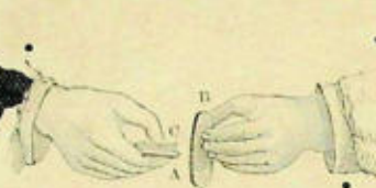
Fig. 5. — Flint and tinder. — The shock of the flint A, against the steel B detaches a fragment of the steel, which becomes red hot, and is known under the name of a spark: it sets fire to the tinder.
