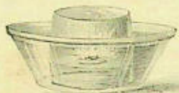
Fig. 16. — Nitrogen remains after the phosphorus by burning has taken up the oxygen of the air.
