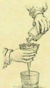
Fig. 26. — The liquid that passes is limpid still, there is in it a little dissolved lime, lime water.
