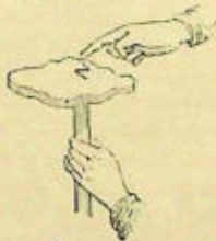
Fig. 64. — I place my finger near it, and I obtain little sparks, and a slight crackling noise.
