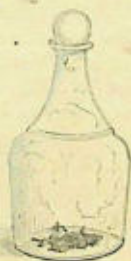
Fig. 111. — The air of the bottle dilated by the heat of the paper has made a vacuum in cooling. — It was then that the atmospheric pressure pushed the egg into the bottle.
