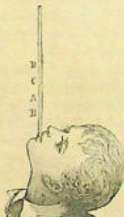
Fig. 16. — The heat of the mouth causes the mercury to rise from C to D.
