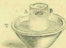
Fig. 117. — The burning paper has produced a vacuum in the glass. This space, the water occupies, being pushed by atmospheric pressure, and mounts as high as AB.
