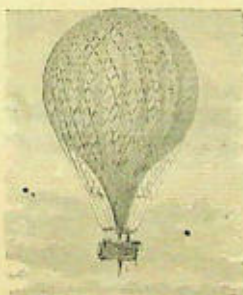
Fig. 13. — Balloons are filled with gas for lighting, which is three times lighter than air.
