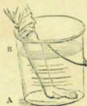
Fig. 109. — You do not feel the weight of 5 lbs because the water weighs equally on all the parts of your hand.
