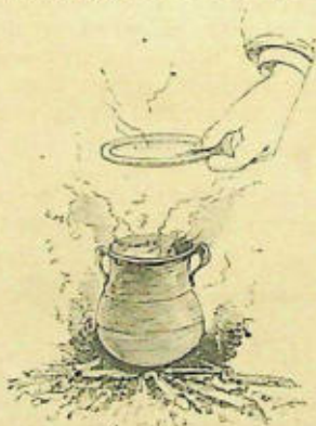
Fig. 7. — The vapour condenses , that is to say, becomes water again, on coming in contact with the cold plate: distillation.
