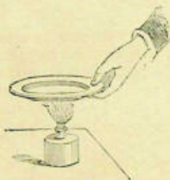
Fig. 15. — The water that condenses on the plate, is the water formed by the combustion of hydrogen that exists in the alcohol.
