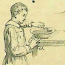
Fig. 93. — The duck is attracted or repulsed according as one or other end of the magnetised needle is presented to it.
