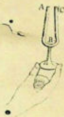
Fig. 55. — Tuning fork. — A, B, C, branch of steel which when set vibrating, gives the la , 806 vibrations in a second.
