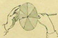
Fig. 46. — The white light is produced by the union of the seven colours of the spectrum.
