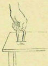
Fig. 87. — The needle is magnetised. Magnetism by contact.
