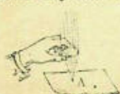
Fig. 42. — All the luminous rays are brought together at the point A, called the focus.
