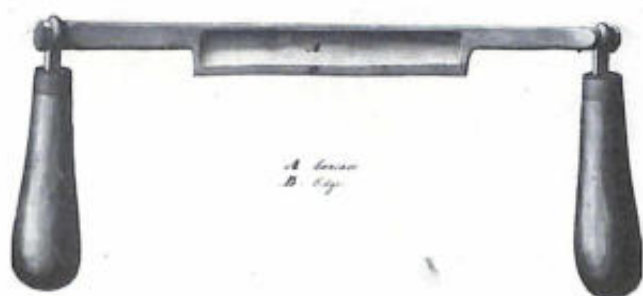
Figure 26.—CONCAVE DRAWING KNIFE patented by Edmund Richards on June 28, 1836 (restored patent 9796X).
