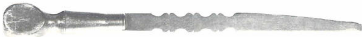
Figure 50.—19TH CENTURY: THE SCREWDRIVER, which began to appear regularly on the woodworker's bench after 1800, did not share the long evolution and tradition of other Anglo-American tool designs. The screwdriver in its early versions frequently had a scalloped blade for no other purpose than decoration. (Smithsonian photo 49794.)
