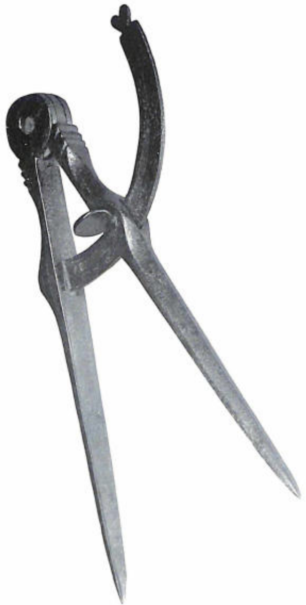
Figure 15.—18TH CENTURY: Cabinet-maker's dividers of English origin. (Private collection. Smithsonian photo 49789-B.)
