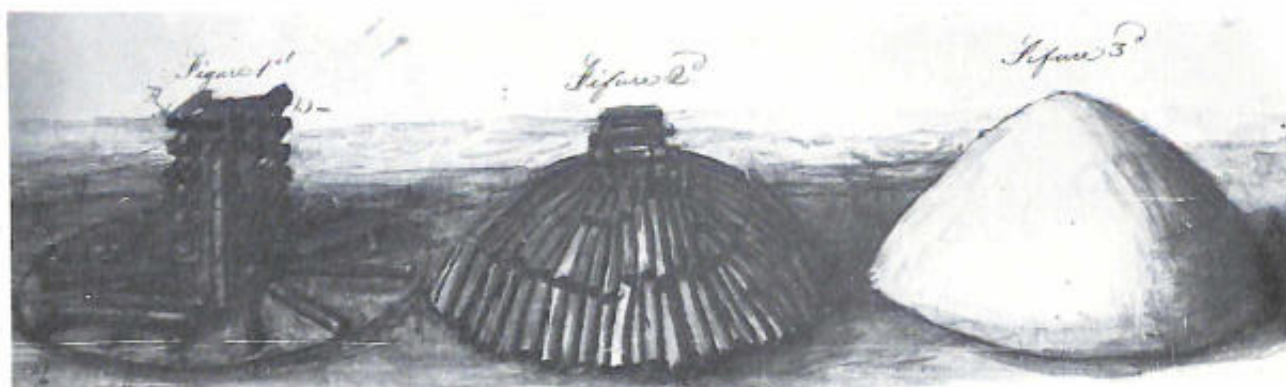
Figure 51.—MODE OF MAKING CHARCOAL invented by Michael Carroll. Patent 720, April 28, 1838.
