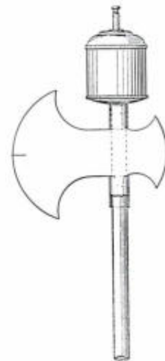
Figure 36.—COMBINED TORCH and battle ax, 1884, as shown in patent 309370, issued December 16, 1884.
