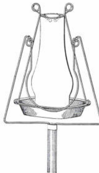
Figure 84.—COMBINED LANTERN AND TORCH, 1897, as shown in patent 585756, issued July 6, 1897.
