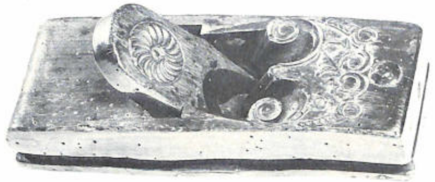
Figure 22.—1756: THE HIGHLY elaborated stock and rosette-incised wedge of the smoothing plane recall the decoration on furniture of the period. The plane is of Dutch origin. (Smithsonian photo 49792-F.)
