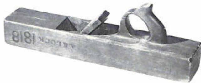
Figure 26.—1818: THE JACK PLANE, used first by the carpenter for rapid surfacing, is distinguished primarily by the beveled and slightly convex edge of its cutting iron. As with the plow and the rabbit, its shape is ubiquitous. Dated and marked A. Klock, this American example follows precisely those detailed in Sheffield pattern books. (Smithsonian photo 49794-C.)
