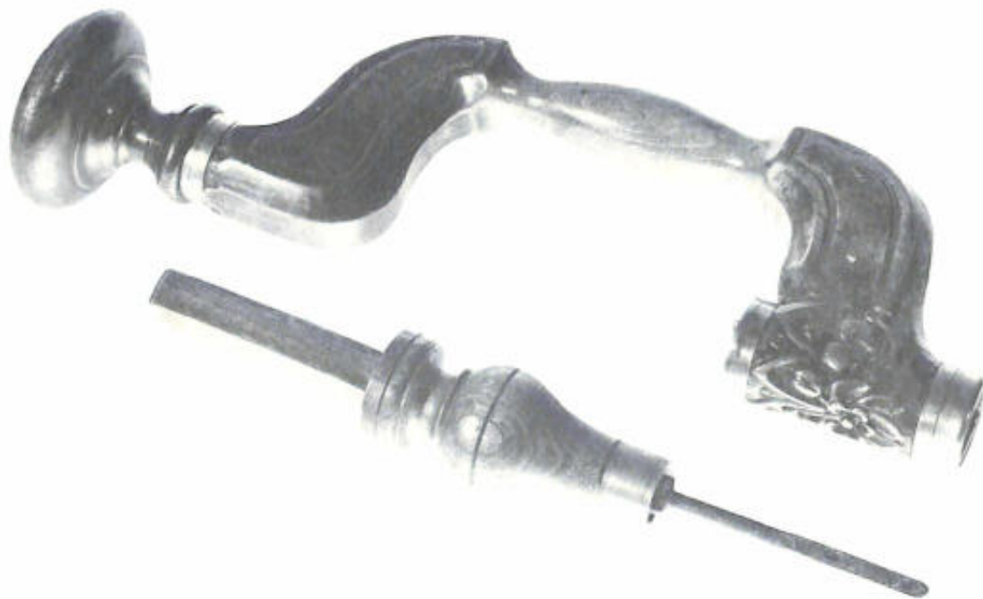
Figure 39.—18TH CENTURY: THE TRANSITIONAL FORM of the wooden brace and bit incorporated the overall shape of the mass-produced version but retained the archaic method of fastening the bit to the chuck. The tool is of Dutch origin and suggests the influence of Sheffield design on European tools. (Smithsonian photo 49792-E.)
