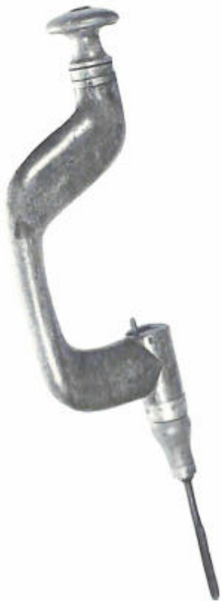
Figure 46.—18TH CENTURY: THE BRACE AND BIT in its nonfactory form conforms to a general design pattern in which none of the components are ever precisely alike. This aspect of variety of detail—sophistication, crudeness, decorative qualities or the like—reflects something of the individuality of the toolmaker, a quality completely lost in the standardization of the carpenter's brace. (Smithsonian photo 49794-A.)
