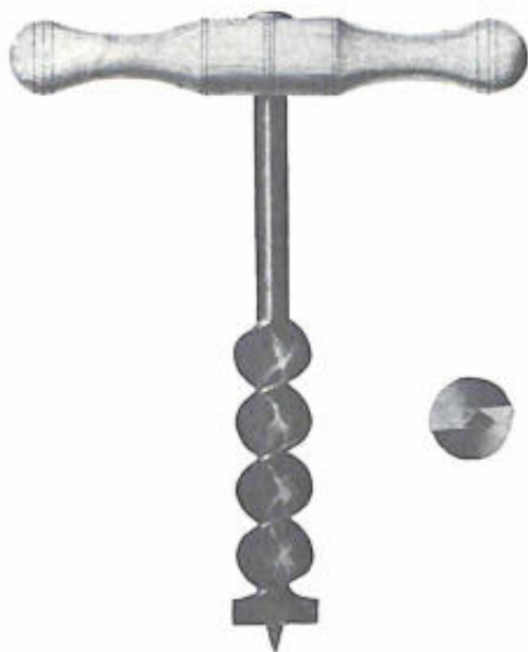
Figure 54.—1809: THE INTRODUCTION of the gimlet-pointed auger followed Ezra L'Hommedieu's patent of 1809. From this date until its general disuse in the early 20th century, the conformation of the tool remained unchanged, although the quality of steel and the precision of the twist steadily improved. (Wash drawing from the restored patent drawings awarded July 31, 1809, U.S. Patent Office, Record Group 241, the National Archives. Smithsonian photo 49790-A.)
