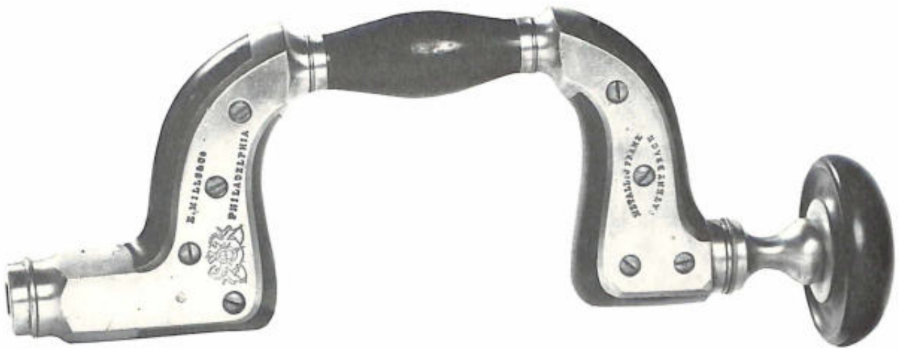
Figure 57.—1876: JAPANNED AND SPLINTED WITH HEAVY BRASS, this brace was among the award-winning tools exhibited at the Centennial by E. Mills and Company of Philadelphia. (Smithsonian photo 49792-D.)
