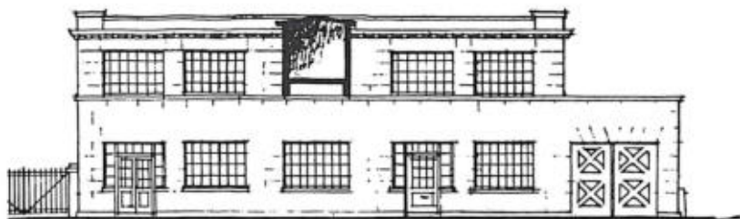
SKETCH OF LOW STRUCTURE PROPOSED FOR THE PUMPING PLANT OF THE AQUARIUM
