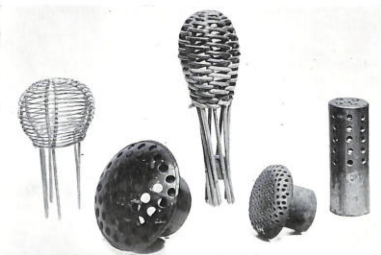
FIVE TYPES OF STRAINERS USED IN THE AQUARIUM TO PREVENT ESCAPE OF SPECIMENS FROM TANKS
