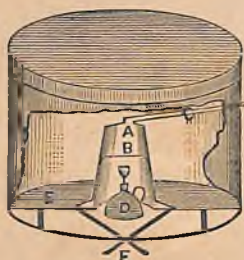
A Heating Cone. B Disc to throw heat to side of Cone. C Air Pipe. D Lamp. E Platform. F Regulator.
