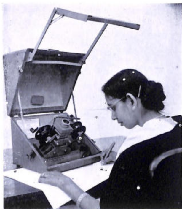
This special type of microfilm reader has the device for throwing the image on a screen for use by a small group. (Courtesy : National Library, Calcutta)
