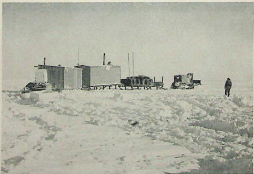
2. A "cat-train" bound for survey operations near Point Barrow. Long hitches of sleds and "wanigans" carry the surveyors, their instruments, and their habitation as a relatively self-sustained unit.
