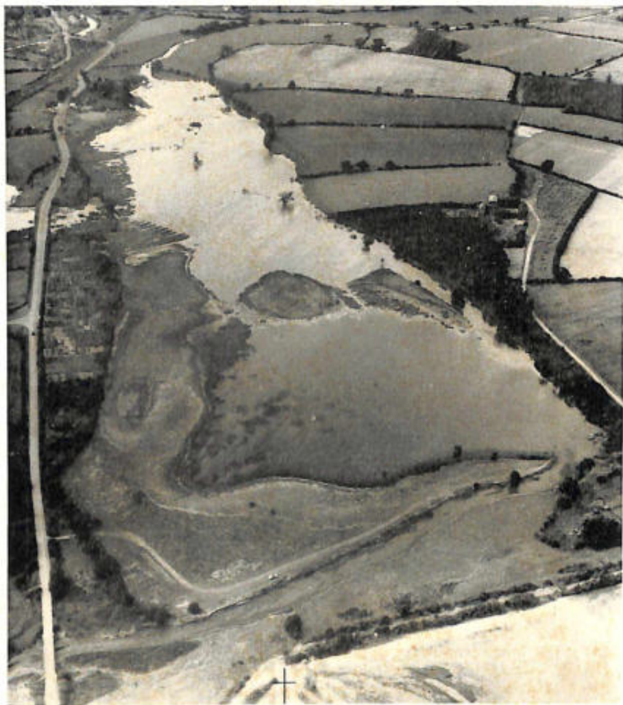
Alvecote Pools, Warwickshire, looking westwards along the extensive flooding resulting from mining subsidence. The pools are a nature reserve and a notable haunt of wildfowl. See page 212
