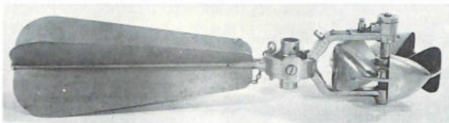
Figure 11.—LARGE PRICE CURRENT METER (24 inches long), model no. 376 in Gurley's early catalogs but no. 600 in later ones. (USNM cat. no. 289642; Smithsonian photo 44538-G.)
