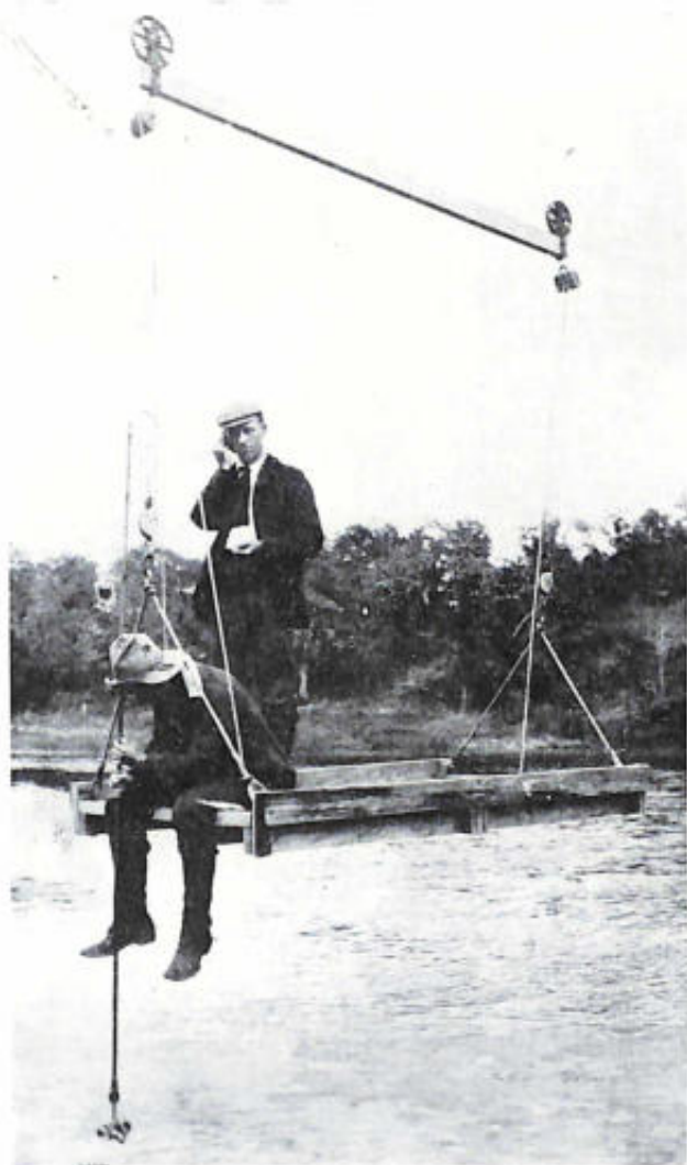
Figure 19.—GAGING CAR provided with blocks and tackles to facilitate using the Acoustic meter. (From U.S. Geological Survey Water-Supply Paper 56, pl. 9.)
