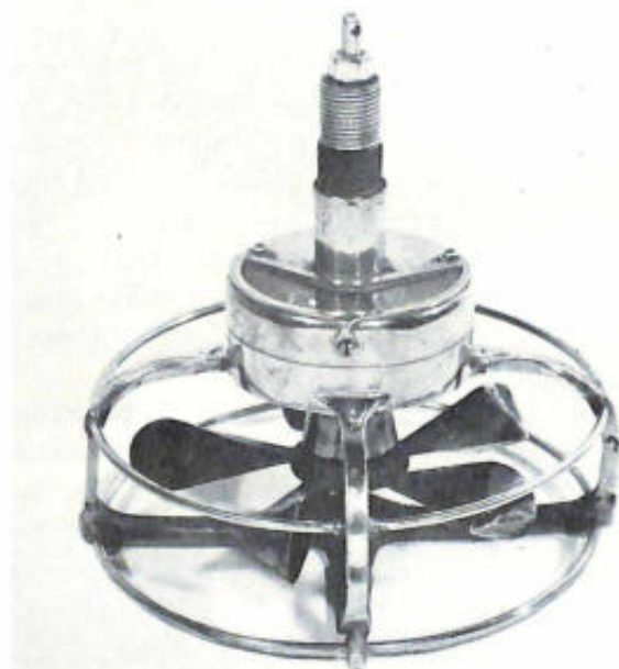
Figure 14.—NETTLETON'S COLORADO CURRENT METER as improved by Bailey of Lallie & Bailey, Denver, Colorado, now in the Smithsonian's Museum of History and Technology. (USNM cat. no. 248696; Smithsonian photo 44538-A.)
