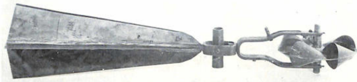
Figure 2.—THE ORIGINAL PRICE CURRENT METER, now preserved in the Smithsonian Institution's Museum of History and Technology. (USNM cat. no. 289638; Smithsonian photo 44538-H).
