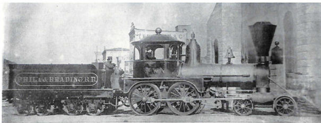
Figure 19.—The Fawn , A LIGHT PASSENGER LOCOMOTIVE built by Millholland in 1860. (Chaney neg. 14479.)
