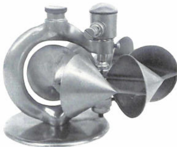
Figure 25.—LATER VERSION of model 618 Small Price current meter. (Photo taken by author.)
