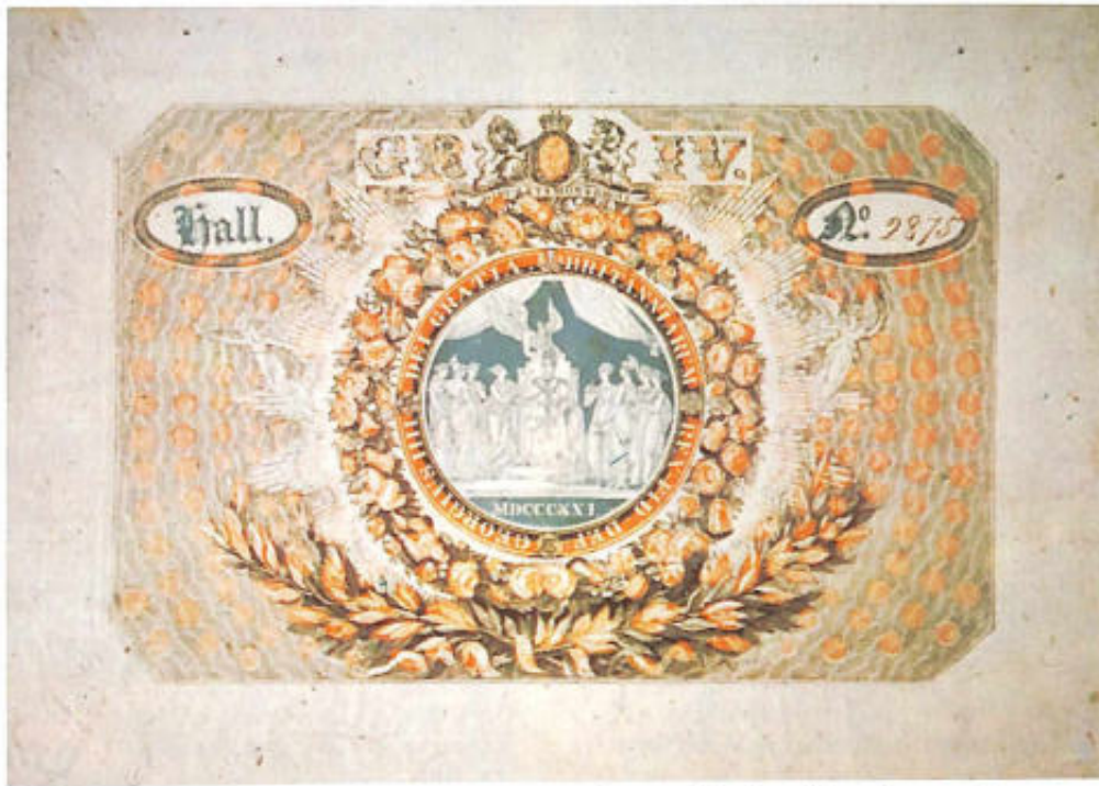
Figure 3.—TICKET TO THE CORONATION OF GEORGE IV printed from Congreve's compound plates, 1821. The border was embossed by Dobbs. Reduced from 5\frac{1}{4} x 8 inches. (Original in Constance Meade Collection, Oxford University Press.)
