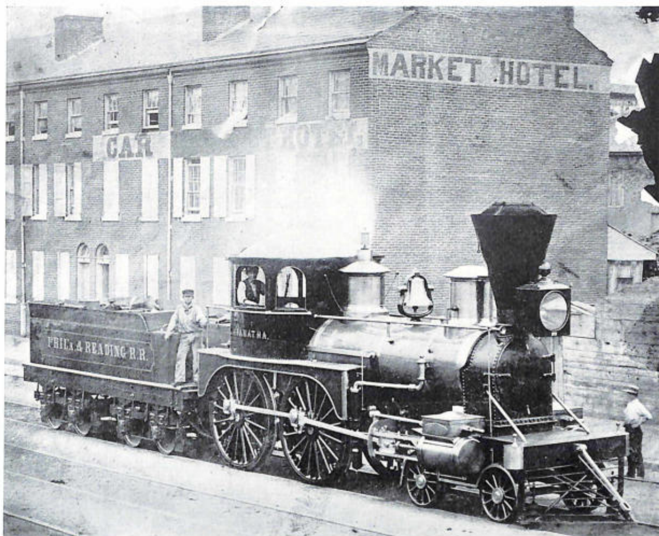
Figure 17.—THIS CLEAN-LINE PASSENGER LOCOMOTIVE, THE Hawatha , WAS BUILT BY MILLHOLLAND IN 1859. It was the first of a very successful class of passenger locomotives and was not retired until 1883. (Smithsonian photo 40630.)
