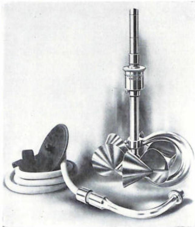
Figure 17.—THE PRICE ACOUSTIC CURRENT METER. (Photo courtesy of W. and L. E. Gurley.)
