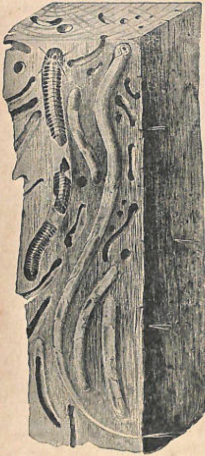
Fig. 933.—Ship-Worms ( Teredo navalis ). A Bristle-Worm has appropriated an empty burrow on the left.
